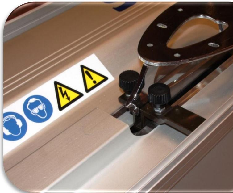
To make the wheel come further away from the toe picks, adjust the screws down.
